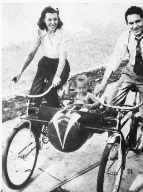
Family-Cycle comes next in chronological order. It's made of two ordinary bikes welded together with a small baby carriage between them. It was built by Roy S. Henrich of St. Louis, Mo.
